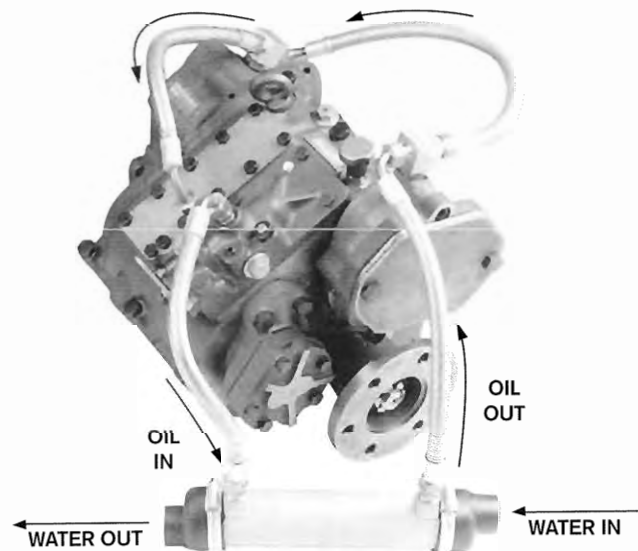
Fig. 13. Oil cooler connections PRM750A/PRM750C with power take-off
